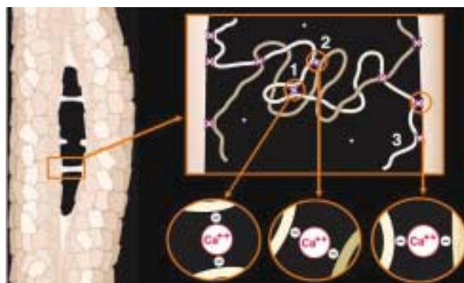
Figure 4. Hypothesized structures of assembled glue molecules, with sacrificial bonds (represented by 'x's) along the backbone of glue molecules resisting rupture of the molecules as they are stretched during microcracking. There are three types of sacrificial bonds, shown in the following order from left to right in the insets: 1) Within one molecule. 2) Between two molecules. 3) Between a molecule and the surface of a mineral crystal. (Modified version of Figure 3 in Fatner et al. Nature Materials 2005; 4:612-616).
